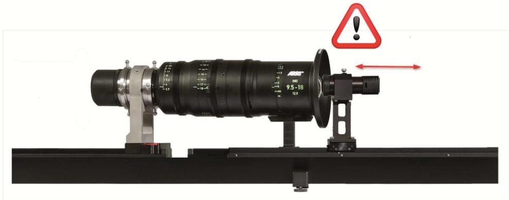
Do not move the projector by hand nor block the projector while it is moving.
